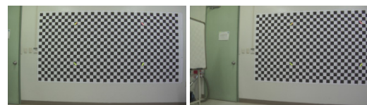
Figure 6. A pair among five of input images used for the calibration of rotational displacement.
